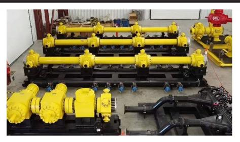
Completion Equipment Rental's Single Line Missile System provides a step change by reducing the number of required connections and providing a single 7-1/16" Single Line system from Frac Blender to Frac Tree. Each high-pressure inlet is configured with a 3-1/16" 15K Flange x 3" 1502 Check Valve.
